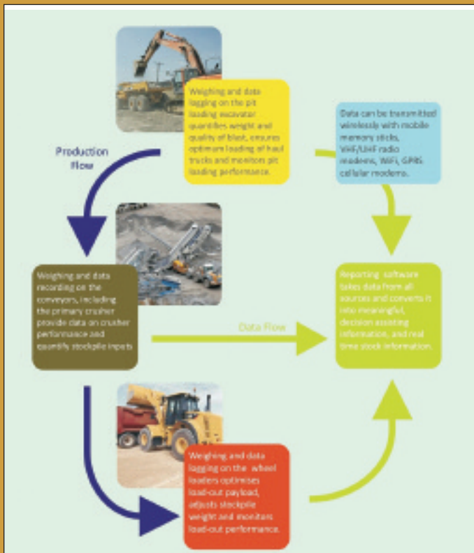
Fig. 1. Principle of Loadrite's Whole Site Solution
