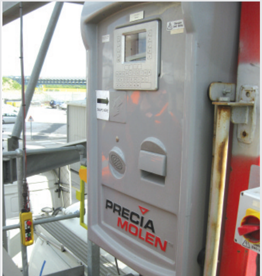
All incoming drivers are asked to input an identification number in the driver console
