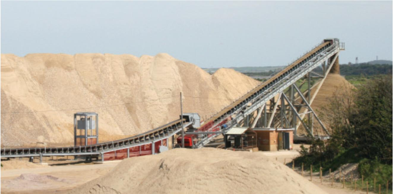
*The new 3,500 tonnes/h ship unloading system at Brett Aggregates' flagship marine aggregates operation at Cliffe, in Kent*
