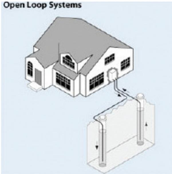
Open-loop ground-source heat pumps could be used to extract heat from groundwater
