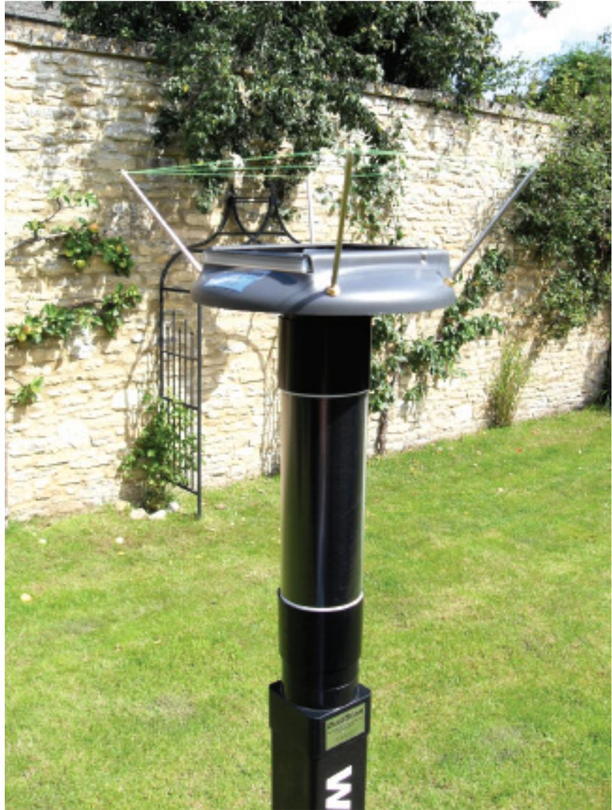
A sticky pad dust-flux monitor; this instrument is also fitted with a dust-settlement gauge
