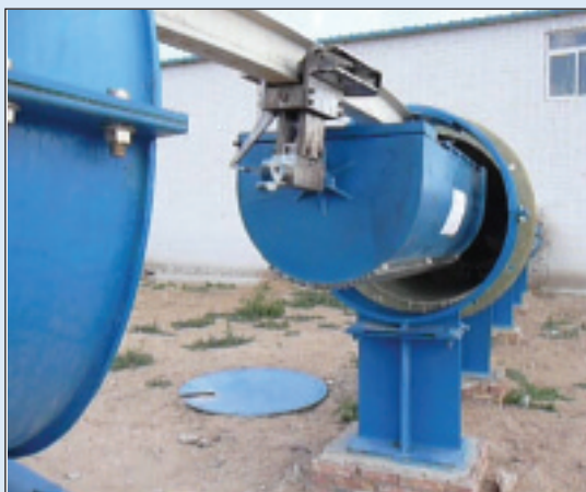
Fig. 5. Capsules for the Magplane Technology coal pipeline suspended from a test track
