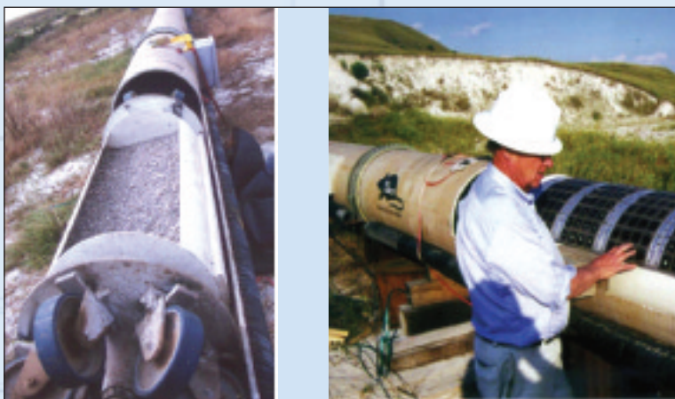
Fig. 4. Magplane Technology demonstrator capsule carrying 300kg of phosphate (left) and the linear synchronous motor (right)
