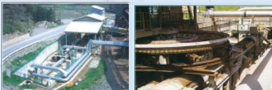
Fig. 3. Aerial view and close-up of the capsule loading area of the Sumitomo Metal Industries capsule system
