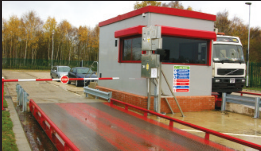
Fully automated weighbridge system
