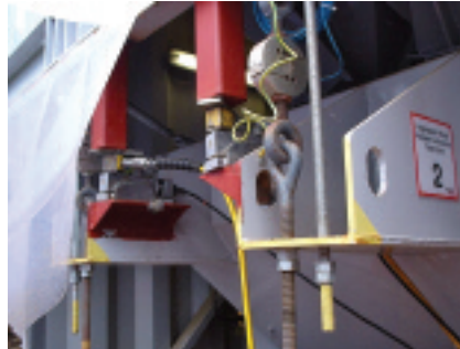
Force calibration of aggregate weigh hopper
