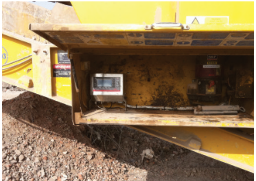
TTCS's FXM belt weigher is connected to this on-board 1400 programmable indicator
