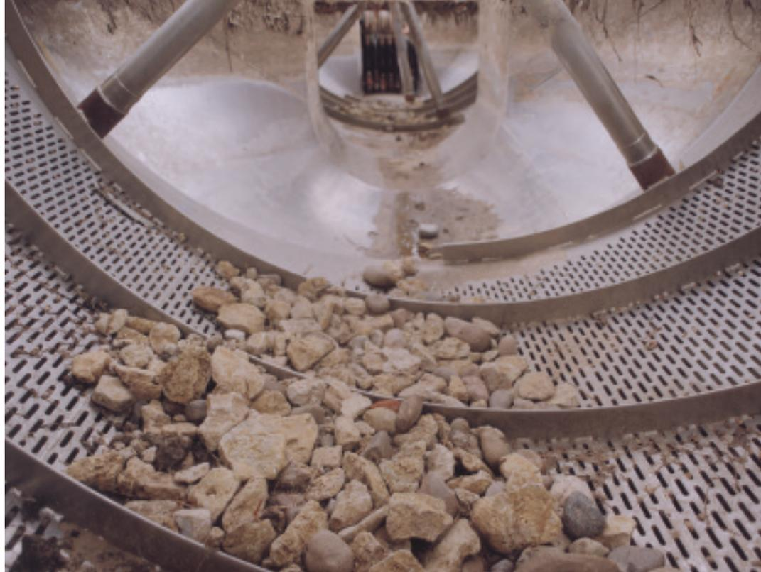
*A rotary screen constructed from 3CR12 stainless steel*
