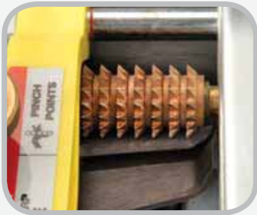
Front drive rollers aggressively grip belt at the start of the skive to prevent slippage.
