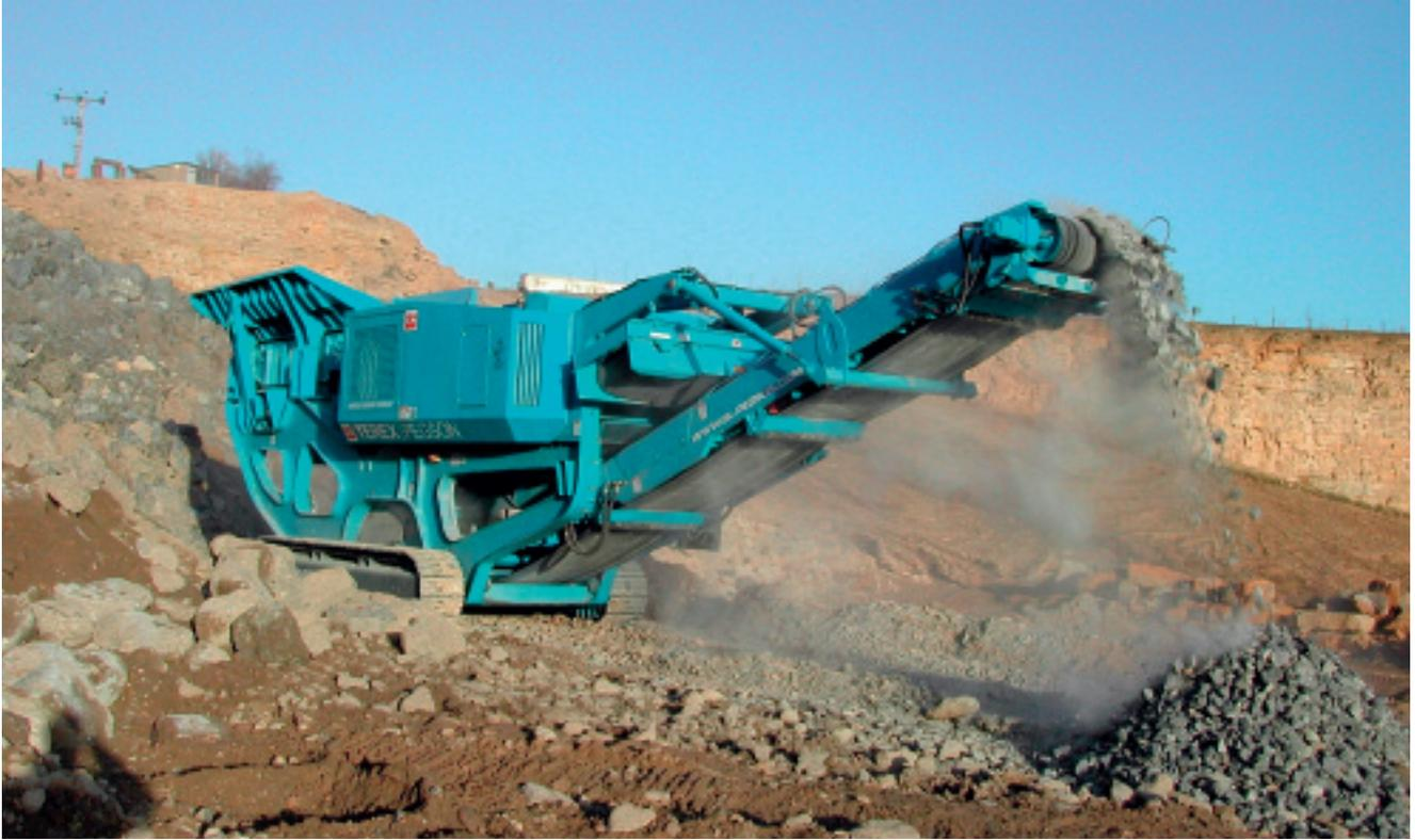
Designed for primary crushing, the new X400 is available in both hydraulic adjust (HA) and hydraulic release (HR) versions
