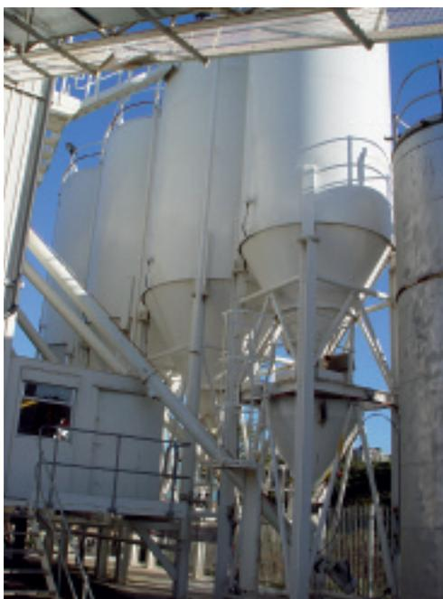
The four cement/dust silos with the plant control room visible bottom left
