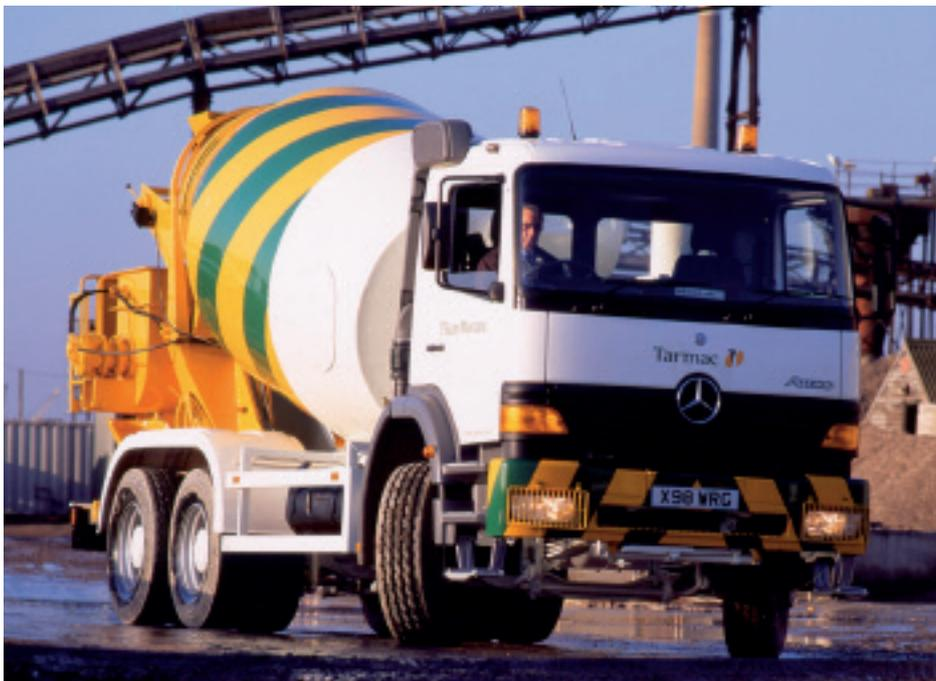
*Mixers are designed and built to produce a mix that is complete and consistent*
